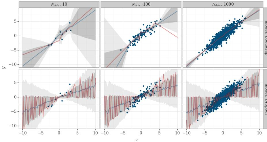
Figure 8: Dropout does not converge with increasing data even with a complex neural network. Grey regions indicate  $\pm 1, 2$  standard deviations, the mean is shown in blue and a single posterior sample in red.
