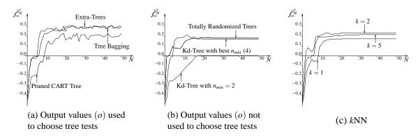
Figure 13: Influence of the supervised learning method on the solution. For each supervised learning method  $\hat{Q}_N(x,-4)$  and  $\hat{Q}_N(x,4)$  are modeled separately. For Tree Bagging, Extra-Trees, and Totally Randomized Trees, the trees are developed completely ( $n_{min} = 2$ ). The distance used in the nearest neighbors computation is the Euclidean distance.
